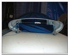
The 'rain risk' position enables airflow identical to that of an open hatch without the inconvenience of rain entering the boat.
